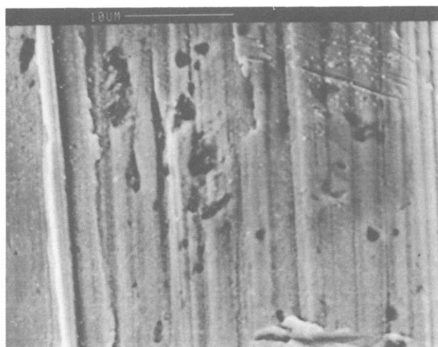
Fig. 6. The alloy on the verge of breaking down with very small corrosion pits forming in wear tracks.
